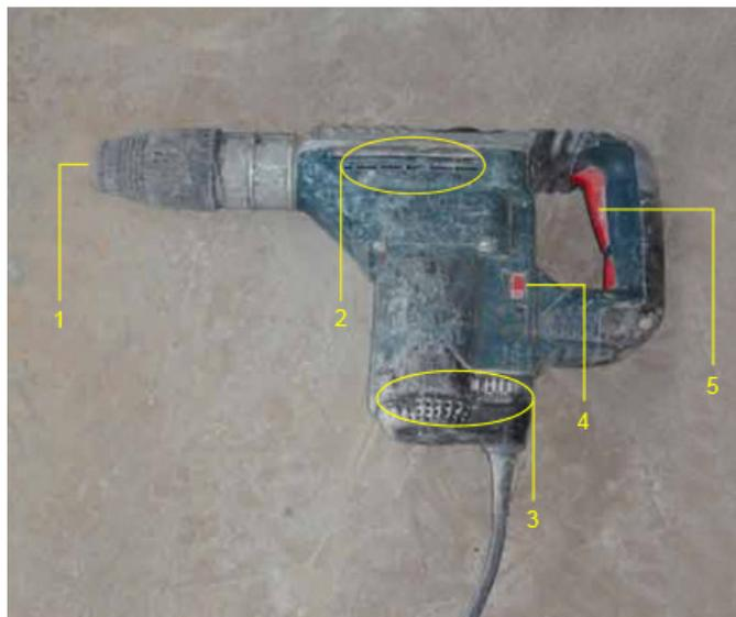
**Figure 6. Marked positions are highly exposed to dust entry.**
